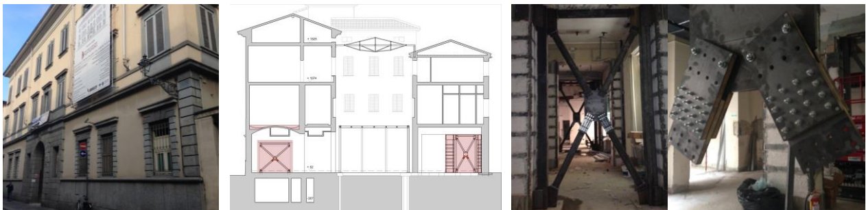
Fig.2 Seismic improvement: (a) Palazzo APE Museo in Parma; (b) cross section of the structure with strengthening interventions; (c,d) brick columns jacketing and Meldamp ® damping system.
